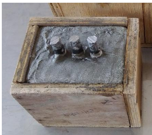
Figure 2. Concrete block with three reinforcing steel bars.
