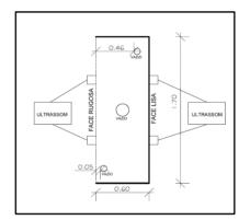
Figure 2. Positioning and depth of voids.
