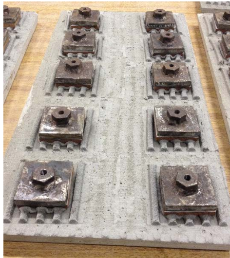
Figure 4. Metallic pieces attached on the ceramic tiles adhered to the substrate-pattern.
