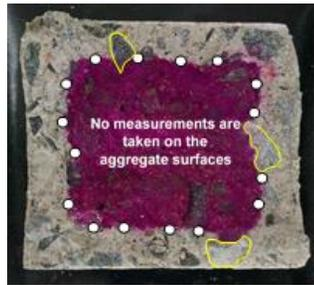
Fracture surface across specimens of 100 × 100 × 500 mm
