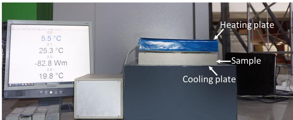
Figure 2. Thermal conductivity test setup.
