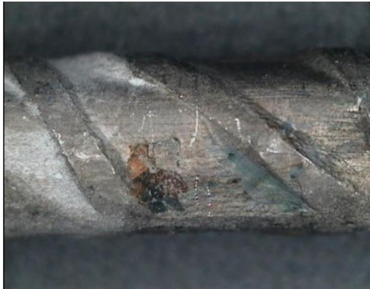
Figure 4. Small spots of corrosion due to chloride attack
