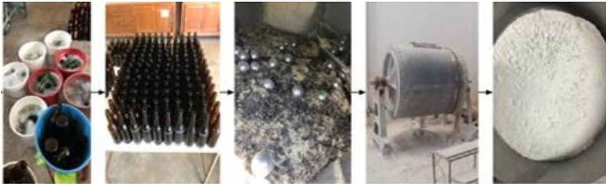
Figure 1. Recycled glass powder processing.
