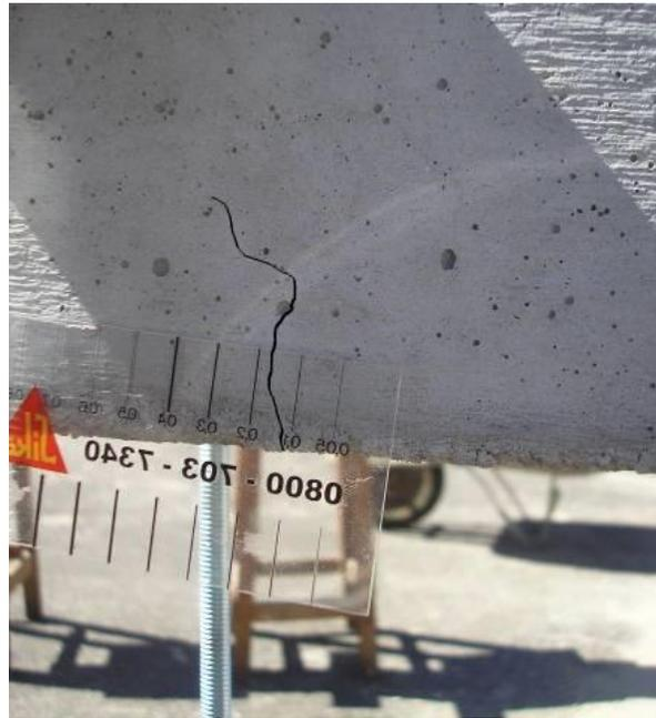
Figure 3. Measurement of the crack opening in the center of the prismatic specimen with a crack meter.
