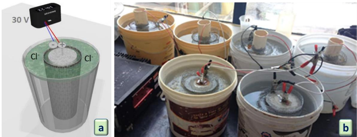
Figure 3. Schematic of the chloride migration test: (a) schematic of the electrical connection; (b) photo of the assembled experiment.
