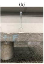
Figure 7. Karsten tubes fixed on the panels: (a) Panel tube without fissure, (b) Panel tube with fissure.
