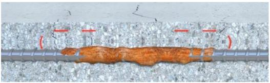
Figure 7. Spalling due to chloride corrosion.
