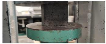
Figure 5. Uniaxial compressive strength (UCS) testing machine for mortars.
