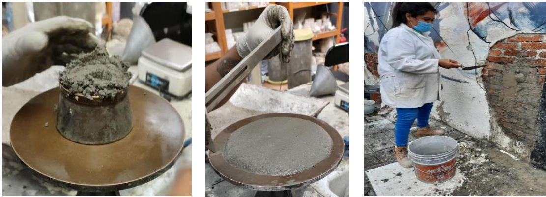
Figure 3. Trials on the mortar mixtures: a) Mixture in mold; b) Consistency; c) Adherence. Image source: (Duran, 2021).
