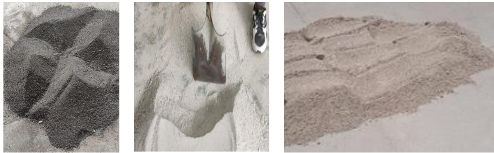
Figure 1. Sand aggregates: a) Joyitas volcanic sand; b) El Coro volcanic silty sand; (c) El Cuervo river sand. Image sources: (Durán, 2021; Durán, 2021; Mondragón, 2021).
