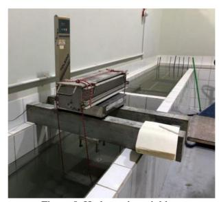
Figure 8. Hydrostatic weighing.
