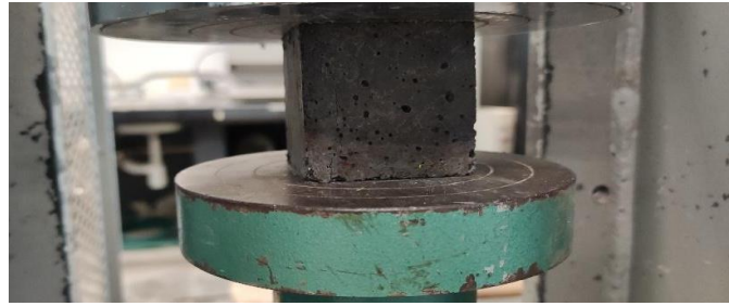
Figure 5. Uniaxial compressive strength (UCS) testing machine for mortars.
