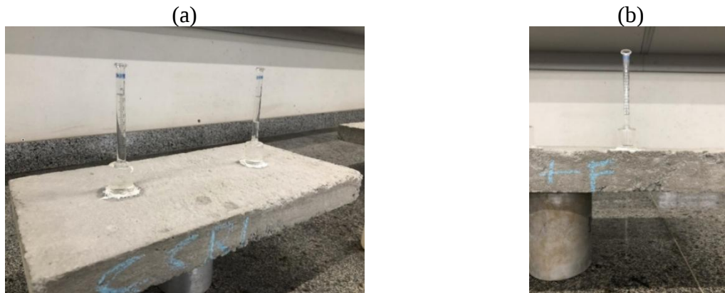
Figure 7. Karsten tubes fixed on the panels: (a) Panel tube without fissure, (b) Panel tube with fissure.
