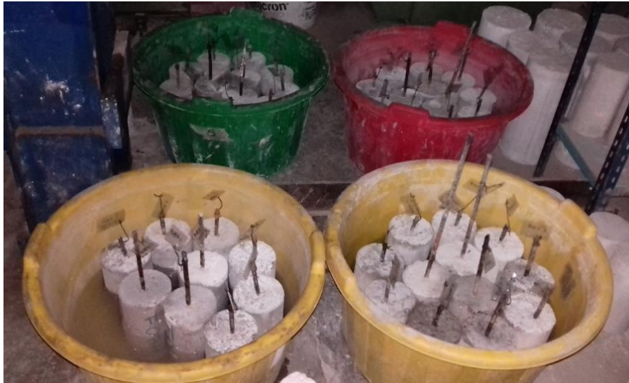
Figure 2. Exposure condition of the specimens to be evaluated.
