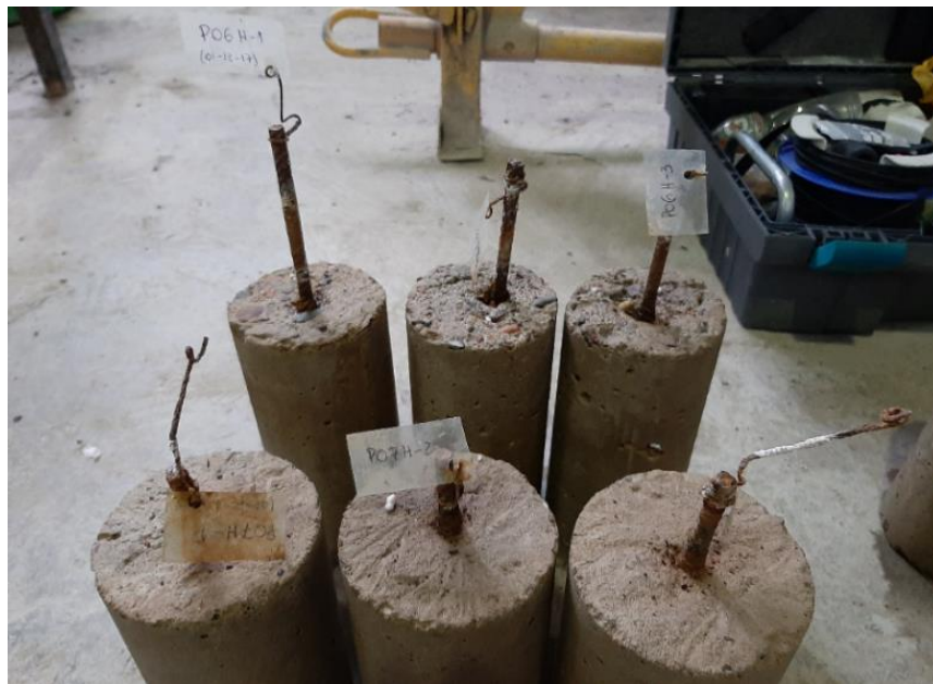
Figure 3. Bar embedded in the upper face of the specimens.
