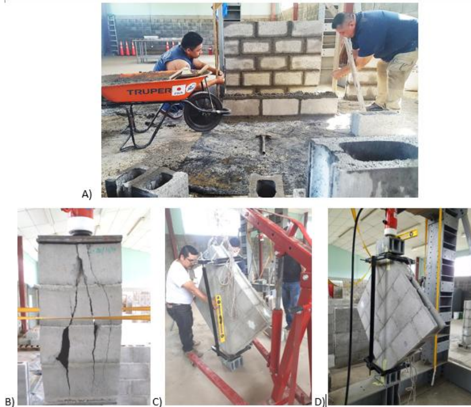
Figure 1. Construction process and testing of prisms and walls.
