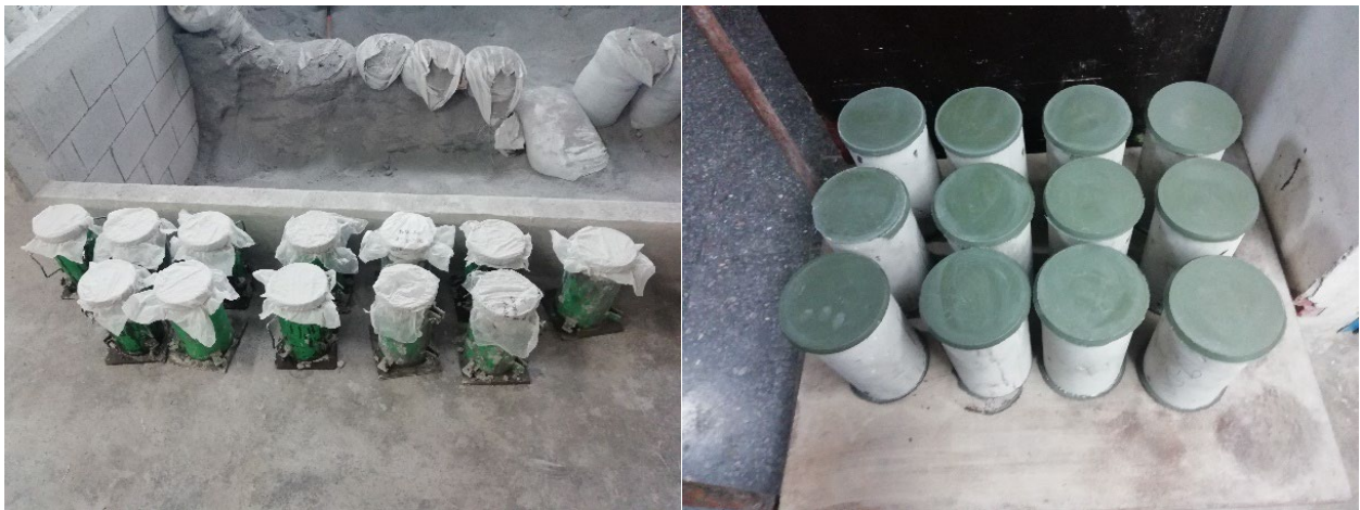
Figure 1. Fabrication and pitching of cylinders 150 mm in diameter x 300 mm in height.
